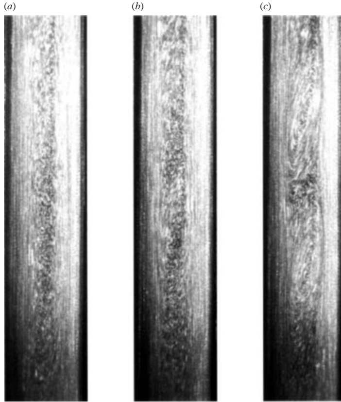
FIGURE 3. Streak images of flow in the mid-section of the tank. (a) Gr = 11\,700 , boundary layer flow; (b) Gr = 13\,000 , transitional flow; (c) Gr = 14\,300 , multicellular flow.
